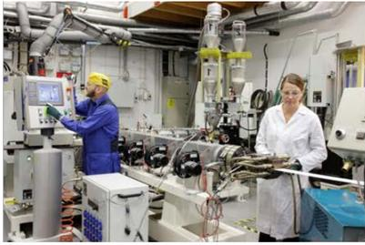
Material and production process development targeting light weight thermoplastic core structures produced in continuous extrusion foaming line
