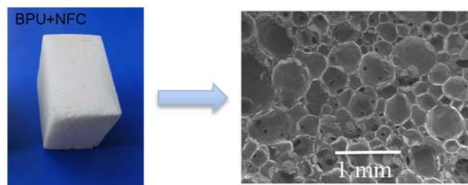
*Biobased polyurethane with nanocellulose fibres*
