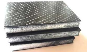
Initial sandwich assembly tests with foamed PLA core
