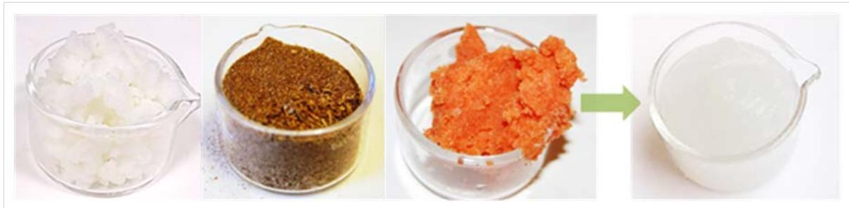
*Illustration of the raw materials: birch kraft pulp, barley residue and carrot residue and the nanofibrillated cellulose obtained after bleaching and grinding*
